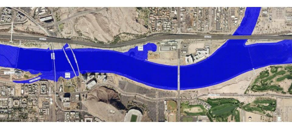
Designed to maintain or improve current levels of flood protection – 210,000 cubic feet per second (cfs.)
